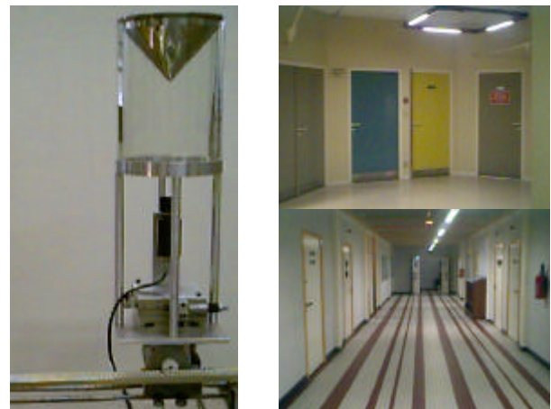
Figure 12 : Our stereoscopic omnidirectional sensor and the two experimental environments
